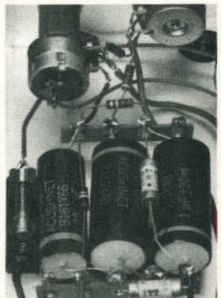
Photo C. Components in the CRT cathode supply are as originally described in the SB-620 manual. Note the long insulated bushing on the INTENSITY control. The piggyback switch is rewired for +12 volts.
